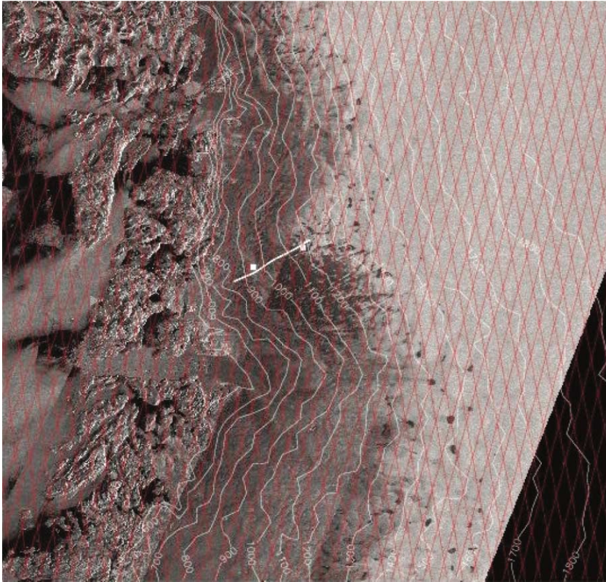
Fig. 2.1. ICESat ground tracks for 183-day repeat cycle overlain on a SAR image (195 km N–S by 205 km E–W) of the ice margin in west-central Greenland along with surface elevation contours (100 m intervals) mapped from ERS radar altimeter data. Location of the U. of Colorado's Swiss Camp ( 69^{\circ} 34.3' \text{ N} , 49^{\circ} 18.2' \text{ W} ) on the equilibrium line at 1170 m elevation is shown in the center. The bare ice in the ablation zone is darker than the firn above the equilibrium line where darker summer-melt lakes are also visible.
